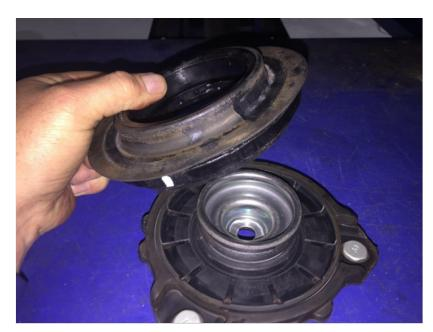
Remove and re-use OE bump-stop and upper spring seat/bearing - these will be re-used with new strut top
