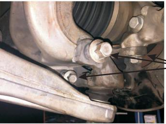
• Un-bolt lower front bushing bolt.
