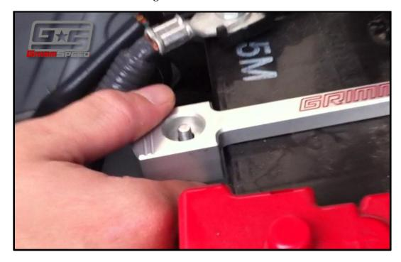
Figure 3: Hook the front j-bolt.
