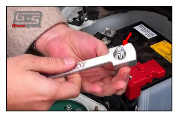
Figure 1: Loosely attach rear j-bolt to the tie down.
