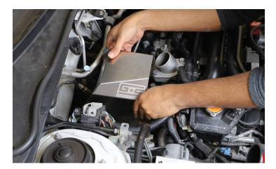
5. Use the included 10mm hardware to secure it in place.
