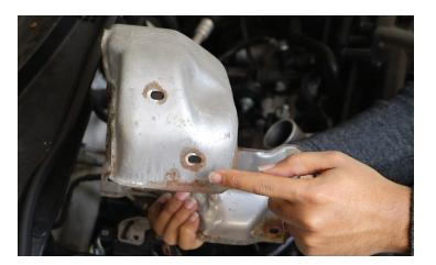
2. Remove the 10mm bolt from the lower heatshield bracket.
