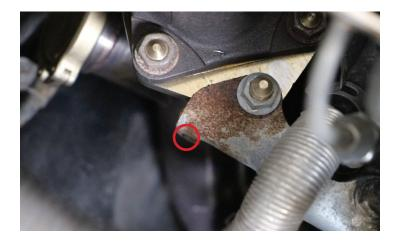
3. Use the top bracket mounting holes to secure your new heat shield.
