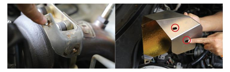
If you have any questions don't hesitate to contact us directly! Support@GrimmSpeed.com | 612-379-0000 4. Place your GrimmSpeed Heat Shield over your turbo and align the mounting holes to the bracket.
