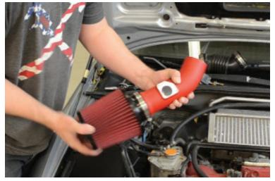
17. Take your heatshield and insert the intake pipe into the hole.
