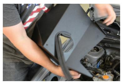
14. Grab the second longest piece of bulb gasket and apply it to the back of the heat shield.
