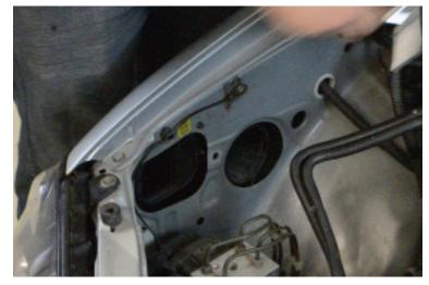
12. From underneath the car remove the other bolt holding the snorkus to the chassis and pull the unit out.
