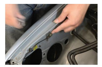
19. Take the whole intake assembly and carefully put it into place. Make sure all the mounting holes are aligned and the heatshield is seated correctly.
