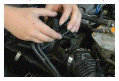
4. Using a flat head screwdriver, loosen the two OEM hose clamps on the stock intake elbow.
