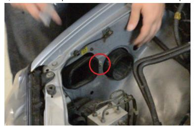
11. Push the snorkus/resonator assembly into the inside of the fender so you can remove it from under the car.
