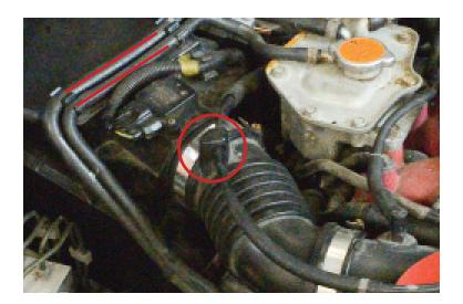
2. Unclip the MAF Sensor connection from the airbox and move it out of the way.
