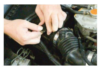
3. Using a phillips head screwdriver, remove the two MAF screws and pull the sensor out.
