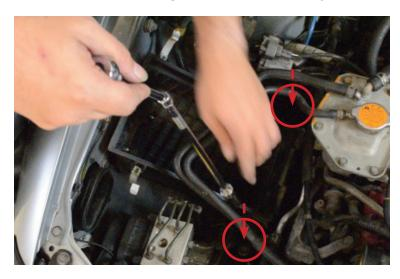
9. Using a 12mm socket with an extension, remove the two bolts and pull out the airbox.
