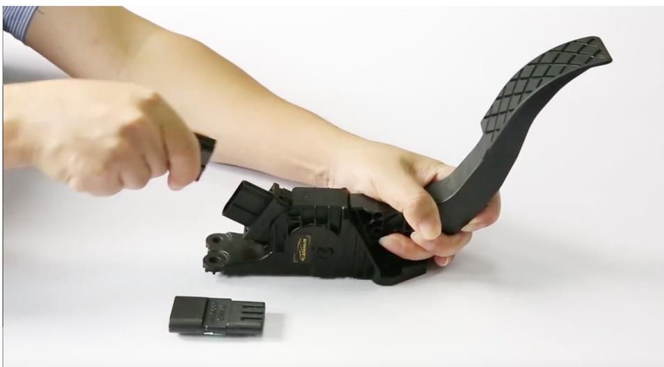
3) Plug the iDRIVE into the top of the pedal assembly.
