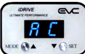
**Automatic Control** – This mode is what makes the iDRIVE unique. AC automatically chooses the Ultimate throttle response based on pedal pressure. If you accelerate gently it will ease it on from 1, If you accelerate hard, it will ramp it up to 9.
