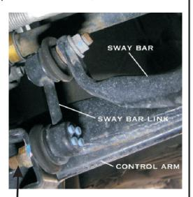
Re-check Ball Joint nuts after 100kms travelled
