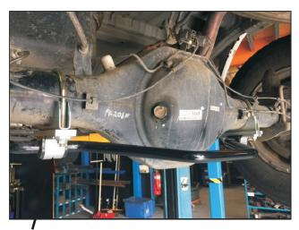
Axle mounting components - U bolts Axle brackets Flat plates D Saddle Flange nuts
