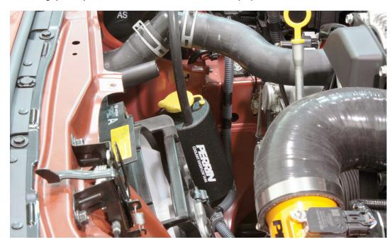
8. After a day of driving it may be normal to see a small amount of coolant come out of top of tank. This is normal as the system is just settling out. Do not keep filling tank beyond half way if you see it drop below half way. This will just push out more coolant in the future.
