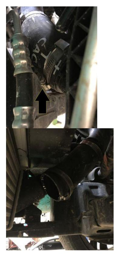
15. Now, we'll want to loosen and remove the entire driver side charge pipe. Do so by using a 7mm socket and loosen and remove all clamps. Pull the piping connecting the intercooler to the throttlebody out and set it all aside. We don't need it anymore.
