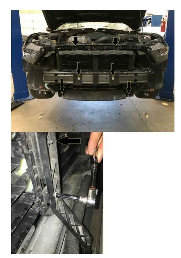
12. With the grill shutters out, we need to remove this cross bar at the front of the frame rails. Use a 10mm socket to remove the four (4) bolts and set the cross bar aside.
