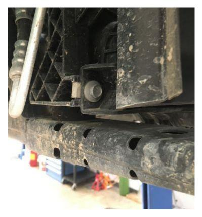
18. Now, on the driver side, there is clip system that you must unclip. From here, you should be able to start getting the intercooler removed. You may need to push back on the radiator, twist in all sorts of strange ways, but eventually, you'll get this FMIC out. Just take care not to damage any fins on the radiator or intercooler in the process. Just be patient, you'll get it!
