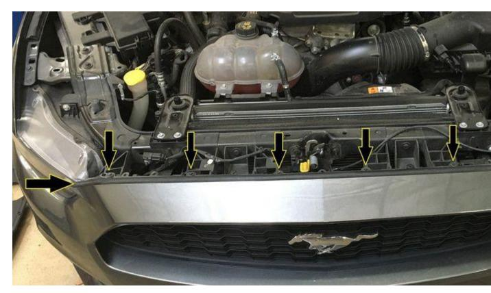
5. Using a 5.5mm socket, remove the two screws that are covered up by the soft trim at the sides of the bumper, near the headlights. These are shown with the horizontal arrows above and further
