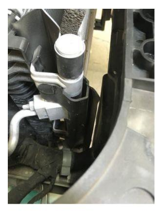
14. With the panels removed, now it's time to finally remove the factory FMIC. Using a 7mm socket and extension, loosen the bottom most hose clamp that connects the passenger side charge pipe to the intercooler and pull it away from the intercooler. Bend it up and out of the way.
