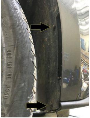
8. Once the fender rivets are removed, you'll be able to pull back the plastic liner to access the single 7mm bolt that is located up at the corner of each side of the bumper. This bolt holds the corners of the bumper to the front quarter panels. This needs to be removed completely on both sides before attempting to remove the bumper.
