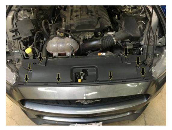
4. Using an 8mm socket, remove the six (6) screws that line the top of the bumper, as seen with the vertical arrows below.
