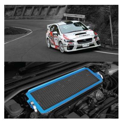
Subaru WRX/STI have always had a top mounted intercooler directly facing the hood scoop, which is highly efficient and easy to service. However, owners frequently are faced with excessive collection of debris in the fins, and cleaning of fins which are extremely delicate.
