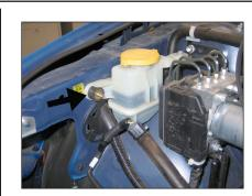
9. Install the provided short, m/m rubber mounted stud into the P/S reservoir as shown.
