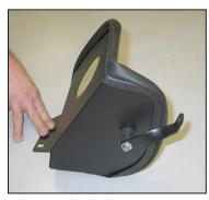
18. Install the heat shield mounting bracket assembly onto the heat shield as shown and secure with the provided hardware.
