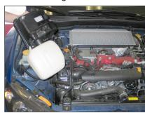
7. Remove the stock air filter housing from the vehicle.
