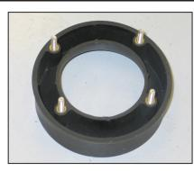
12. Install the four 6mm studs into the filter adapter as shown.
