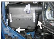
6. Remove the bolt and nut that secure the stock air filter housing.
