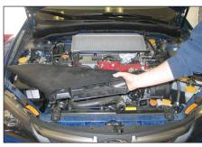
3. Remove the two clips that retain the fresh air inlet duct. Then remove the fresh air inlet duct from the vehicle.
