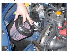
15. Set the filter assembly into the fender in preparation for the heat shield installation.
