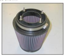
13. Install the filter adapter assembly into the K&N® air filter and secure with the provided hose clamp.
