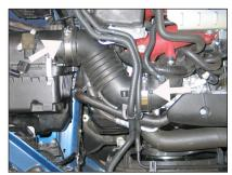
4. Loosen the two hose clamps that secure the stock intake tube.
