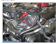
11. Install the provided silicone hose (08421) onto the turbo inlet and secure with the provided hose clamps.
