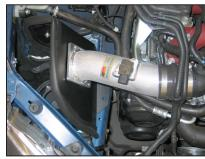
22. Install the K&N® intake tube into the silicone hose at the throttle body as shown.
