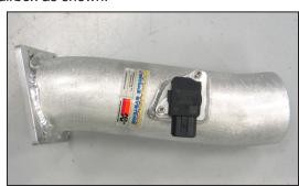
21. Install the mass air sensor into the  $K\&N^{\mbox{\scriptsize 0}}$  intake tube and secure with the provided hardware.
