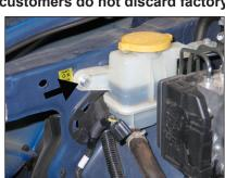
8. Remove the front P/S reservoir mounting bolt shown.
