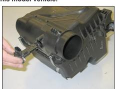
20. Remove the mass air sensor from the stock airbox as shown.
