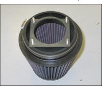
14. Install one of the provided gaskets onto the filter adapter as shown.
