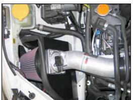
17. Install the K&N<sup>®</sup> intake kit so that the heat shield rests on the rubber mounted studs installed during step #7. Secure the heat shield with the provided bardware. Slide the silicone has onto
