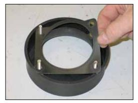
12. Install the filter adapter gasket onto the four studs as shown.
