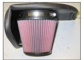
15. Install the K&N<sup>®</sup> air filter onto intake assembly and secure with the provided hose clamp. NOTE: Drycharger<sup>®</sup> air filter wrap; part # RU-5147DK is available to purchase separately. To learn more about Drycharger<sup>®</sup> filter wraps or look up color availability please visit http://www.knfilters.com<sup>®</sup>.
