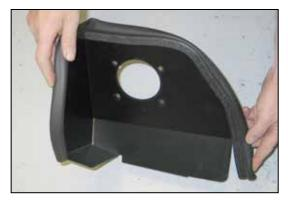
10. Install the provided edge trim onto the heat shield as shown.
