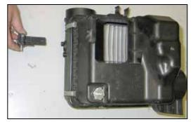
2. Remove the two fasteners which retain the fresh air inlet scoop and then remove the fresh air inlet scoop from the vehicle as shown.
