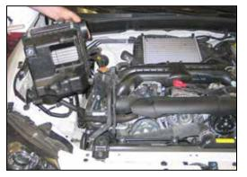
6. Remove the airbox assembly from the vehicle. NOTE: K&N Engineering, Inc., recommends that customers do not discard factory air intake. 8. Remove the two screws which secure the mass air sensor and then remove the mass air sensor from the airbox as shown.
