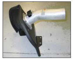
14. Install the K&N<sup>®</sup> intake tube onto the studs and secure with the provided nuts and washers.
