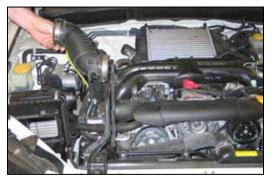
4. Loosen the two hose clamps which secure the factory intake tube and then remove the intake tube from the vehicle.
