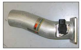
9. Install the mass air sensor into the K&N<sup>®</sup> intake tube and secure with the provided hardware.
