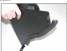
16. Install the provided edge trim onto the heat shield and trim as shown.
