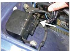
11. Unclip the wire harness from the bracket as shown.
