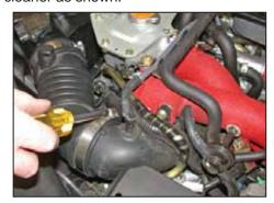
4. Loosen the hose clamp as shown.
