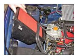
9. Remove the lower air cleaner assembly as shown.
