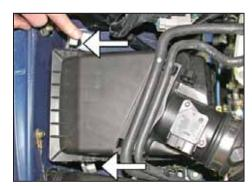
5. Unclip the upper air cleaner assembly as shown.
