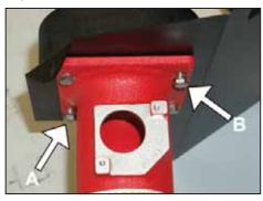
14. Assemble the intake tube, gaskets, heat shield, and filter adapter using the provided hardware as shown.
