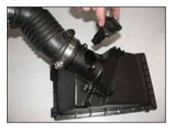
7. Remove the mass air sensor from the upper air cleaner assembly as shown.
