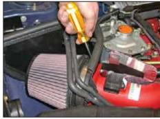
29. Install the K&N $^{\!0}$  air filter and and secure with the provided hose clamp as shown.
