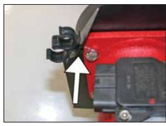
20. Install the hose clip from step 19 onto the heat shield as shown.
