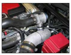
29. Install the bypass valve with silicone hose onto the K&N® intake tube and secure with the provided hose clamp.
