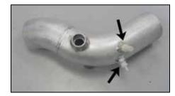
16. Install the two ¼"NPT fittings onto the K&N® intake tube as shown.
