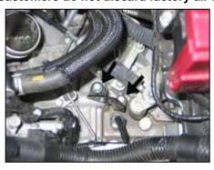
11. Remove the two bolts which secure the transmission/engine lifting bracket and remove the engine lifting bracket from the transmission.
