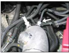
22. Connect the factory vacuum line to the  $\frac{1}{4}$  NPT fitting as shown.
