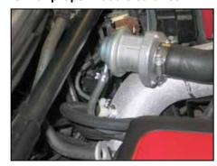
30. Reconnect the factory vacuum hose to the bypass valve and secure with the factory hose clamp.
