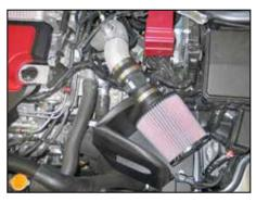
26. Install the mass air sensor assembly onto the K&N® intake tube and secure with the provided hose clamp.
