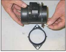
13. Remove the factory gasket and the two spacers from the mass air sensor.
