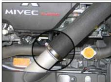
3. Loosen the hose clamps, which secure the upper intercooler hose to the turbo outlet and intercooler inlet.
