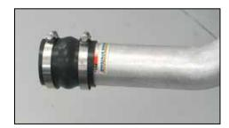
32. Install the remaining silicone hose ( 08487) onto the K&N® upper intercooler tube as shown, slide the hose completely onto the tube and do not secure at this time.
