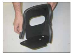
18. Install the provided edge trim onto the heat shield as shown.
