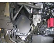
20. Install the heat shield assembly onto the factory air box mounting location and secure with the hardware provided.
