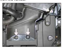
9. Remove the two plastic retaining screws and air box retaining bolt which secure the fresh air scoop as shown.
