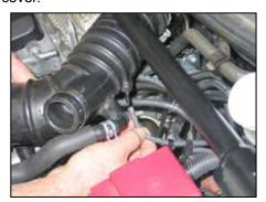
8. Loosen the hose clamps which secure the intake tube to the turbo inlet and mass air sensor. Remove the intake tube partially out of the vehicle and then disconnect the remaining vacuum line. Once the vacuum line is disconnected the complete intake hose assembly can be removed from the vehicle.
