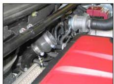
31. Install the silicone hose (08486) onto the turbo outlet and secure with the provided hose clamp.
