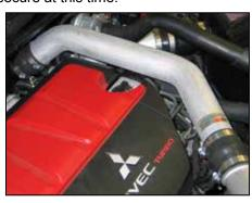
33. Install the K&N® upper intercooler tube into the silicone hose on the turbo outlet, align with the intercooler inlet, slide the silicone hose onto the inlet and then secure with the provided hose clamps.
