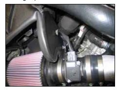
35. Clip the mass air wiring harness onto the heat shield and then reconnect the mass air sensor electrical connection.
