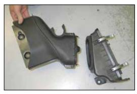
14. Open the air box halves and then push the fresh air intake scoop out of the front air box half.
