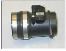
24. Install the provided silicone hose (084031) onto the mass air sensor and secure with the provided hose clamp.
