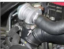
6. Loosen the hose clamp securing the bypass valve to the intake tube and then disconnect the bypass valve from the intake tube, set it to the side.
