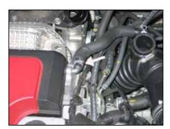
7. Loosen the spring clamp which secures the crank case vent hose to the valve cover and then disconnect the crank case vent hose from the valve cover.
