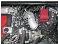
21. Install the K&N® intake tube onto the turbo inlet and align with the mounting bracket installed in step #15. Secure the intake tube with the provided hose clamp and hardware.
