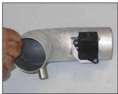
20. Install the mass air sensor into the K&N® intake tube with the provided hardware as shown.
