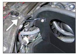
18. Swing the heat shield bracket up under the core support, then mount to the core support using the provided hardware as shown.
