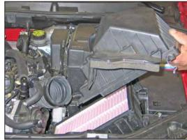
6. Remove the upper airbox housing from the vehicle as shown.
