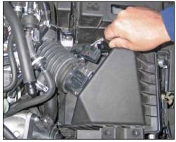
3. Disconnect the mass air sensor electrical connection as shown.
