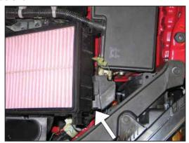
9. Remove the retaining clip, then slide the rubber airbox mount backwards as shown.
