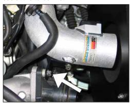
25. Align the intake tube mounting bracket with the solenoid valve, install the provided spacer under the mounting bracket, and secure with the provided hardware. Tighten the hose clamps at the turbo inlet.
