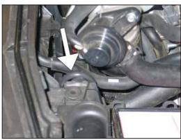
10. Unhook the rubber band that secures the airbox as shown.
