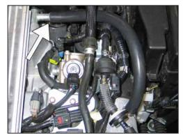
26. Install the provided crankcase vent hose onto the intake tube. Connect the open end to the crankcase vent port (on the engine) as shown.
