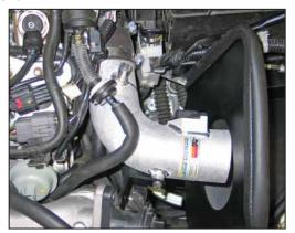
24. Install the K&N® intake tube into the silicone hose at the turbo inlet.
