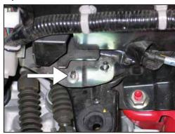
15. Install the provided spacer onto the inner wiring loom stud as shown.
