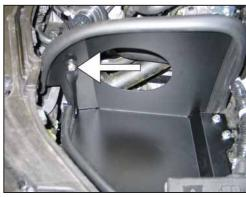
17. Install the heat shield mounting bracket (07945) onto the heat shield with the provided hardware. NOTE: Do not tighten the mounting bracket at this time.
