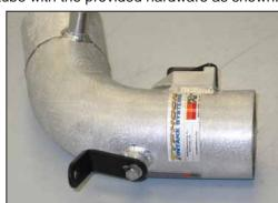
21. Install the tube mounting bracket (#07804) onto the  $K\&N^{@}$  intake tube with the provided hardware as shown.
