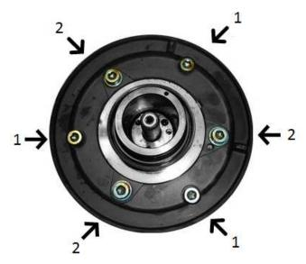
There are 2 bolt sizes that hole the AVCS sprocket together. Below are their tightening torques.
