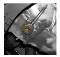
2. For 07 WRX STI with a 6sp manual transmission that utilize a torx T70 transmission drain plug: Remove and install drain plug using the Company23 Torx T70 socket. Bolt torque is 44 Nm (4.5kgf-m, 32.5 ft-lb)
