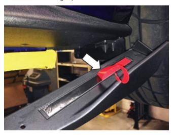
Reinstall the winglet and line it up with the previously marked holes. Install the rear selftapping mounting screw with a 7 mm socket. Torque to 1.0 Nm.
