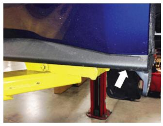
Spread the factory rear rocker trim piece apart from the rocker panel and insert the rocker winglet into the opening until it is fully seated.
