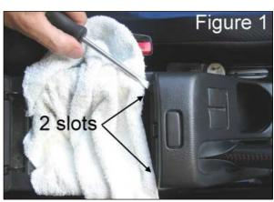
gearstick shroud up from the back, it is only lightly clipped in and does not need much force.
