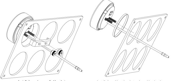
Installation using supplied bracket
