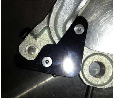
11. Install the Ball Stud with nylon washer into the desired position using a 10mm wrench and a drop of Loctite. The position closer to the factory ball stud is 30% reduction and the next hole is 40% reduction. Please Note: Shift effort will increase with the reduction amount.
