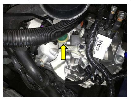
8. Using the marker, make several lines on the top of the shift weight that cross over to the pivot point so that you can realign the weight upon reinstallation.
