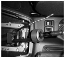
Cable removed from lever
