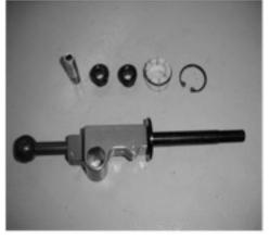
Bushing components to be re-installed
