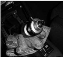
Driving the lockout pin out
