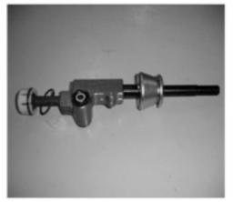
Bushing and trim components on the COBB Tuning Short Shifter
