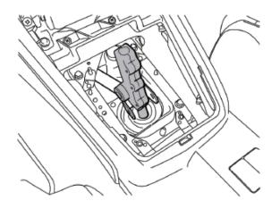
3. Before attaching to the shift linkage, apply a small amount of grease to both sides of the bushings used in the new shifter. There may be enough extra on the ball or socket to use.
