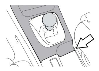
2. Use the two 12mm boxed end wrenches, one on either side, remove the bolt that holds the shift lever to the shift linkage as shown in the picture below. Do not misplace the nut and bolt, as they will be reused with the COBB Tuning Shift Lever.
