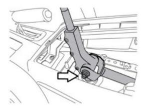
5. You may want to take the time to remove the metal surround that holds down the rubber gasket. Remove the four 10mm bolts and maneuver it out of the car. Trim the upper left edge where the linkage goes by to allow more clearance for the linkage, as it will be slightly higher to get the geometry for a shorter throw.
