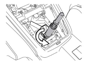
4. Remove the sleeve and bushings from the barrel of the factory lever. These will be reused with the COBB Tuning lever.
