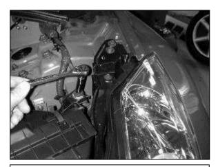
f. Remove the bolt holding the air filter housing assembly in place.
