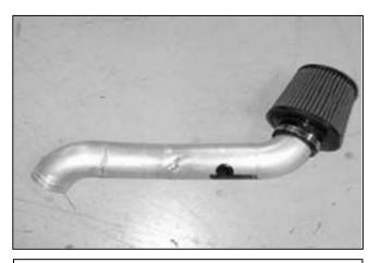
j. Install the air filter onto the end of the lower intake pipe closest to the 7/8" hole. Install the recessed plastic plug in the hole in the intake pipe.
