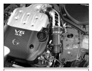
e. Place the 3" silicone coupler around the MAF sensor, not the AEM® MAF adaptor. Connect the assembly to the upper intake pipe. Use the #52 hose clamp around the throttle body and the #48 hose clamps for the 3" diameter tubing. Do not tighten the hose clamps.
