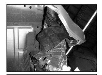
n. It is now possible to gain access to the area behind the front bumper. This is where the air filter will be located.
