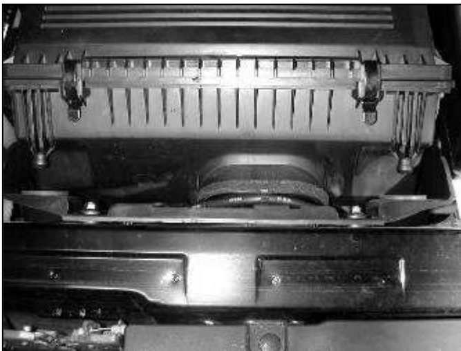
i. Gently pull up on airbox, do not completely remove.
