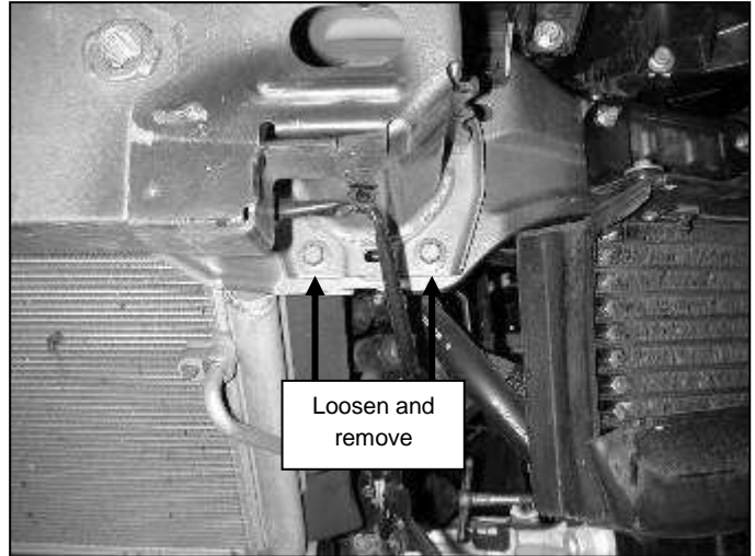
Aj. Loosen and remove the lower two mounting bolts, unplug the temperature sensor and remove the bumper support.
