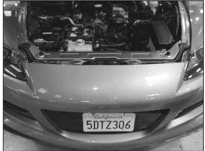
Ab. Remove the bumper and set aside.
