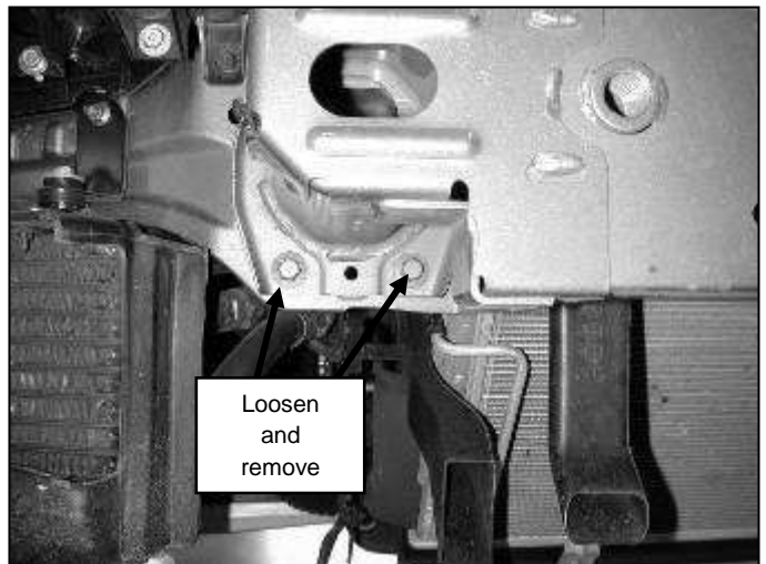
Ah. Loosen and remove the two lower mounting bolts.
