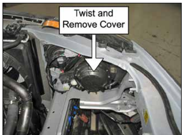
j. Remove the headlight access cover by twisting it counter clockwise. Save the cover for later use.
