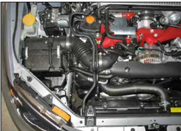
Factory air box system installed
