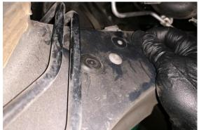
Using 14mm and 10mm wrenches, secure the fuel filter bracket to the chassis, as shown.
