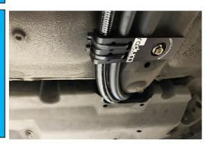
Near the fuel filter, secure the fuel lines using the provided cable zip ties. For LHD vehicles, pay close attention to the steering arm.
