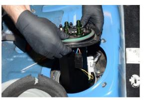
19. The top plate and gasket should be flush with the mounting ring.
