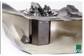
$20. \ Install \ the \ OEM \ metal \ hold-down \ bracket \ and \ tighten \ all \ nuts \ to \ factory \ spec \ in \ an \ alternating \ cross-pattern.$
