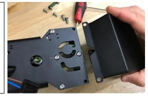
15. Remove the last four M5 bolts on the backside using a 3mm Allen hex wrench. This will detach the 2 fuel pump clamps from the assembly, as shown.
