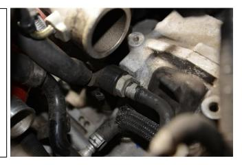
12. Remove the hose barb fitting from the intake manifold.
