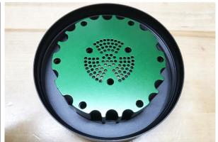
3. Apply a high strength thread locker and secure all 9 included button head bolts using a 5/64" Allen hex wrench.
