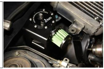
22. Remove each hose from each valve cover vent port (right side and left side).
