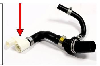
28. Using needle nose pliers, carefully pull to dislodge the small metal jumper shunt (shown) inside the PCV leak detection diagnosis connector. It is not a resistor.
