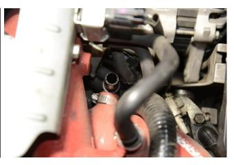
27. Some late model Subaru vehicles will have an electrical connector tube (shown) on the OEM hose that routes to the turbo inlet pipe.
