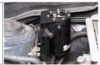
19. Attach the 28" heater hose to the coolant manifold nipple from step 13.
