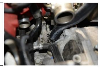
15. Prepare the AOS-R for installation. First, lubricate the O-ring on the 8AN male fitting with light oil. Next, fully tighten the fitting into the side port.
