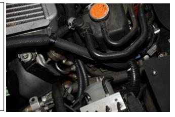
25. Use the remaining  $\frac{1}{2}$ " PCV hose to make a connection between the left side valve cover vent port and the other branch of the Y-fitting. Cut the hose to length (roughly 36").
