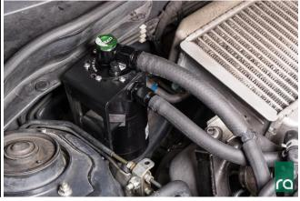
24. Fully insert the plastic Y-fitting into the 5/8" PCV hose, as shown. Use a section of the included %" PCV hose to go from one branch of the Y-fitting down to the right side valve cover vent port. Cut the hose to length (roughly ~13") and secure to the vent port using the factory spring hose clamp.
