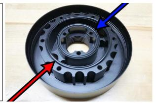
2. Place the green coolant seal plate on top of the O-rings. This CANNOT go on upside down but it goes on in a VERY specific orientation. The outer fins and all 9 bolt holes should align perfectly, as shown.
