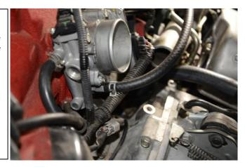
21. To attach the AOS-R side "vent" port to the turbo inlet pipe, measure and cut the  $\frac{1}{2}$ " PCV hose (it will be roughly ~23"). Next, attach this  $\frac{1}{2}$ " PCV hose to the nipple on the turbo inlet pipe and secure with the factory clamp.
