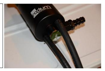
18. Once properly clocked, the AOS-R can be bolted to the bracket. Using a 3mm Allen wrench, tighten the seven included M5 bolts to the AOS-R.
