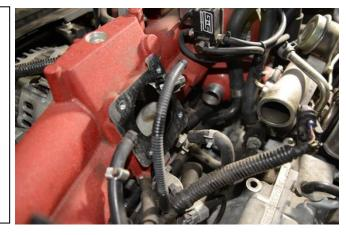
11. Locate the PCV valve fitting underneath the turbo compressor. Remove the small hose going to the intake manifold.
