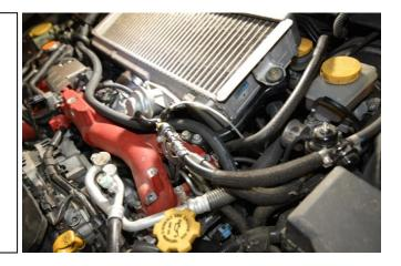
26. Remove the OEM valve cover vent hose from the air intake pipe.
