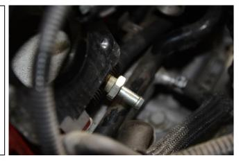
13. Remove the PCV fitting and the small section of rubber hose from the port on the engine block, as shown in RED.
