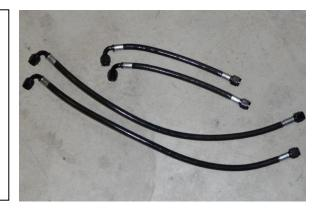
16. 2000-2005 S2000: Find the 2 SAE quick connect male to -6AN male adapter fittings in the kit. Using a vice, install these fittings to the straight hose end side of each of the short hoses as depicted.
