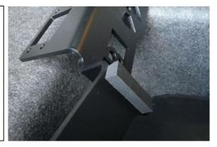
11. Position the Radium Engineering bracket so that the 3 studs from the isolation mounts line up to the corresponding holes.
