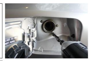
6. To release the gas filler tubes from the chassis, use a 10mm socket wrench to remove the M6 bolt shown.
