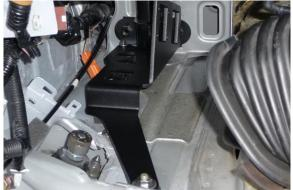
12. Before securing the FST to the bracket, confirm the FST is clocked so the fuel pump pickup is at the lowest point in the FST.
