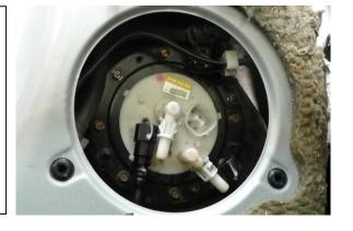
15. 2000-2005 S2000: The 2 short hoses and 2 long hoses will connect strategically to the FST. The short hoses connect to the OEM tubes previously disconnected from the fuel pump hanger. The long hoses will connect to the OEM fuel pump hanger.
