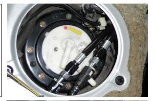
18. The next step is important. The "FST fuel pump outlet" fitting on the FST needs to connect to the OEM tube which routes to the fuel rail. This is the tube that connected into the side port of the fuel pump hanger. For 00-05 kit (shown), this is the green fitting. For 2006-2009 kit, this is the fitting that comes out of the side of the FST-R.
