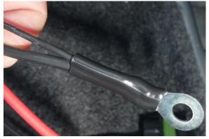
28. The FST pump's relay trigger will be tapped from the OEM fuel pump's yellow/green strip power wire.
