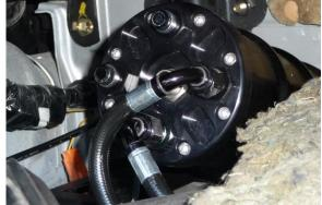
19. 2000-2005 S2000: Find the 2 SAE female adapter fittings in the kit. Install these fittings to the straight hose end side of each of the long hoses as depicted.
