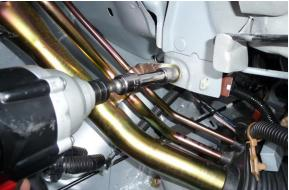
7. From the trunk area, pull the gas filler inwards to release the 3 studs from the body.
