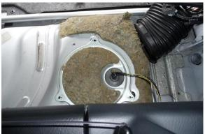
14. The center port on the 2000-2005 S2000 fuel pump hanger is the drain back from the FPR back to the OEM tank. The other port (shown lower right) connects the OEM pump to the fuel rail. Note: The 2006-2009 S2000 only has this fitting.
