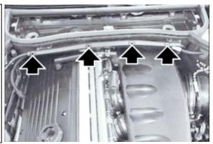
5. Unscrew four T30 Torx bolts (1) and remove lower section of micro filter housing (2) by pulling towards the front of vehicle.
