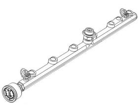
14. Before inserting the fuel injectors into the Radium fuel rail, clean and lubricate all O-rings with clean oil.
