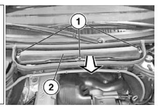
4. Unclip the 4 tabs (shown) for the cable duct in front of the cowl and separate the two long pieces.
