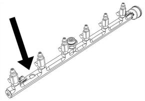
16. For 2005-2006 models that have a PCV solenoid mounted on the vacuum rail, slightly pry the 2 mounting tabs (shown) back ~1mm as they may come in contact with the top of the rail.
