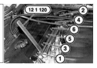
9. The vacuum rail must also be removed from its seat. For this, it is NOT necessary to remove the large brake booster hose.
