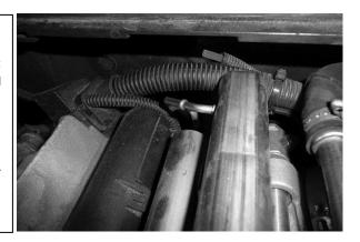
7. Because the new big bore fuel rail takes up more space, the barbed nipple will need to be slightly modified.
