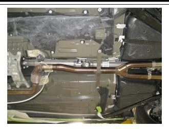
**Step 2.** Begin installation of the new system by loosely attaching the Y-Pipe Assembly to the outlets using the OEM clamp. Leave all clamps loose until final adjustment.
