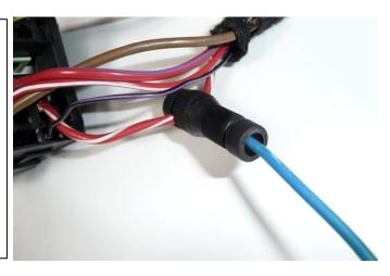
6. To properly use crimpless solder butt connectors, strip the wire insulation back and insert a wire through one side and then twist the 2 wires together. Next, center the connector on the bare wires and use a heat gun to melt the solder. Be careful with the surrounding area as the internal solder can take awhile to melt. Finally, verify the connection is solid by gently tugging.
