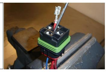
3. It is recommended to connect the "TRIGGER" wire to the ECU fuel pump relay output which has a fuel pump priming attribute and a safety feature which disables the output typically when engine speed is 0 RPM.
