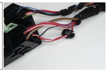
4. Screw the center section back on making sure the OEM wire gets pierced.Next, strip the blue insulation of the relay wire back to expose 3/8" of copper.Slide the opposite end of the Posi-Tap connector over the blue wire, as shown.Insert the blue wire through the center section of the Posi-Tap connector.
