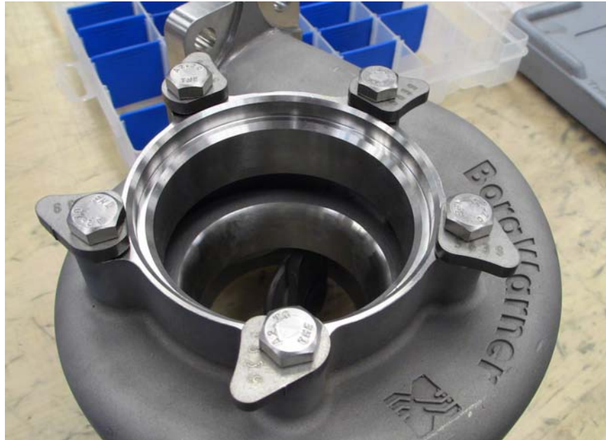
Figure 72: Turbine Clamp Plates Swiveled Out of the Way to Allow Bearing Housing Installation. Clamp Plates Face with Numbers Up.
