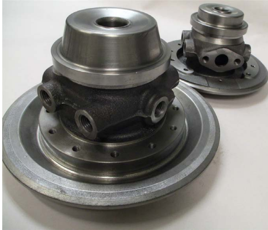
Figure 35: Series EFR Bearing Housings, B1 (back) and B2 (front)
