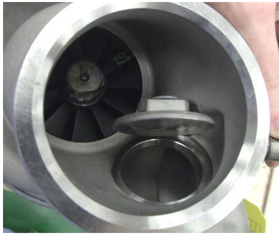
Figure 16: Large Internal Wastegate
