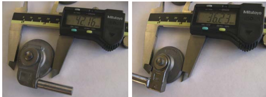
Figure 17: Wastegate Valves - 36mm and 42mm
