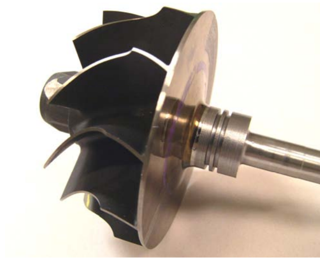
Figure 38: Gamma-Ti Shaft and Wheel Assembly (Superback + Fullback)
