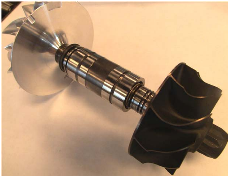
Figure 37: Best of Both Worlds; Ball Bearings + Gamma-Ti Turbine
