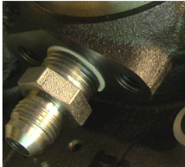
Figure 78: Another Picture of Dual-Machined Oil Outlet Flange (either for gasket or fitting)
