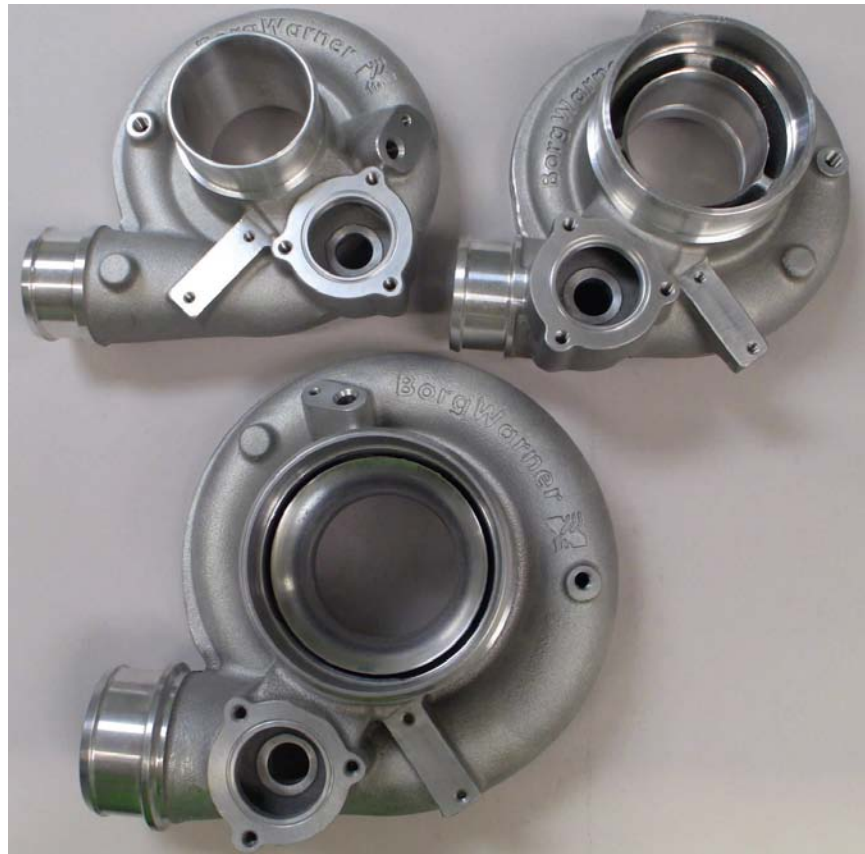
Figure 79: Compressor Covers and Their Inlets and Outlets
