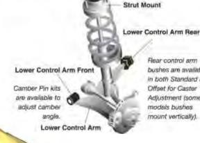
Rear control arm bushes are available in both Standard & Offset for Caster Adjustment (some models bushes mount vertically).
