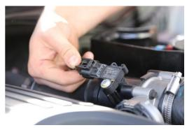
Loosen the screw holding the factory fitted MAP sensor in place. Ensure that this screw is kept in a safe place.
