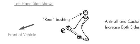
*Note:* Polyurethane bushes must be fitted to both sides of the vehicle.
