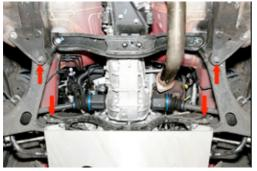
We suggest putting your cars up on ramps to install the front underbody suspension brace, as load on the suspension makes the install go easier.
