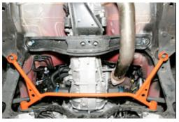
Torque all the bolts down to factory specs. After you've let the car down and driven it around for about 100 miles, check that the bolts are all still at the correct torque setting.
