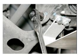
Next, unbolt the front bolt and nut from each lower arm. The suspension will hang down slightly at this point, further if it's on a lift or jacks.
