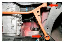
Slide the bolts through the front on both sides first (top arrow), as that is the most difficult part of the installation. Then slide the bar down over the bolts at the rear.
