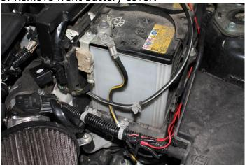
4. Line up the left grommet hole with the existing front battery cover hole near the top of the cover. The bracket grommets should be parallel with the top of the front battery cover.
