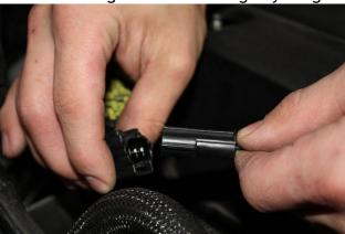
10. Hook up vacuum lines. Port 1 on the GrimmSpeed BCS will connect to a high pressure boost source. Connect the 4mm (smaller) vacuum line from the wastegate to Port 1 of the BCS.
