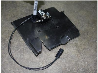
5. Drill the left side mounting hole using a 1/4" drill bit.
