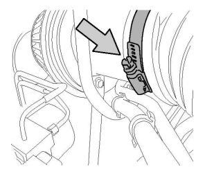
6. Make sure to plug in the MAF sensor connector. It can go above or below the intake as well.
