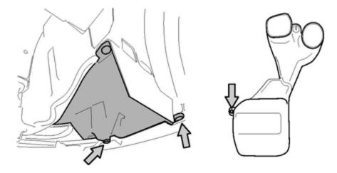
11. Place the splash guard back in it's original position and reinstall the pop-in retainers.
