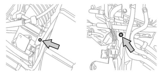
7. Use the phillips head screwdriver to remove the MAF sensor from the factory airbox. BE VERY CAREFUL WITH THE SENSOR AS IT IS SENSITIVE AND CAN BE DAMAGED.
