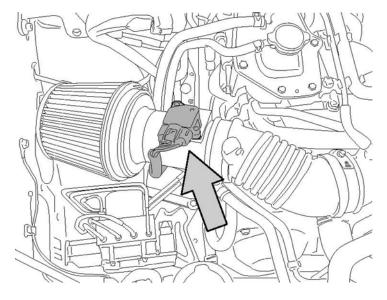
5. Position the COBB SF Intake in a manner which closely matches the stock MAF sensor orientation. Assure that it does not contact the ABS system, strut tower, fender, or the wheel well. Tighten the mounting bolts to secure the COBB SF Intake into position. Tighten the clamp that secures the intake hose to the COBB SF Intake. Make sure that it is fully inserted.
