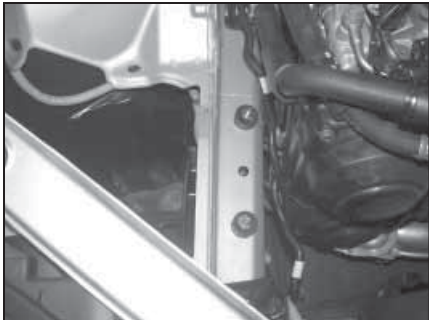
18. Install the provided rubber mounted studs into the original air cleaner mounting holes as shown.
