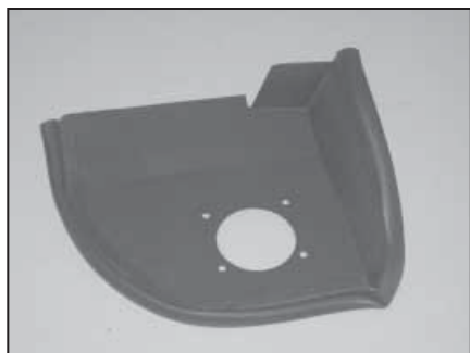
11. Install the trim seal onto the heat shield and trim to fit if necessary.
