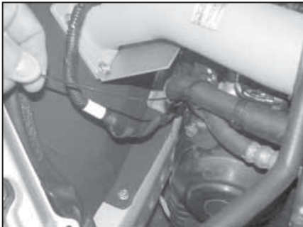
24. Zip-tie the coolant hose and power steering hose together as shown.
