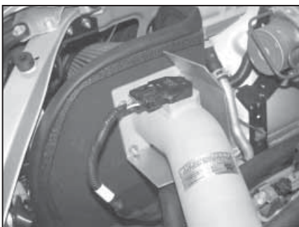
23. Reconnect the mass air sensor electrical connection as shown.
