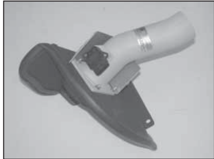
16. Install the heat deflector plate onto the tube flange and secure it with two nylock nuts and flat washers as shown.
