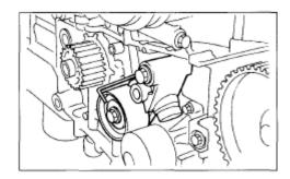
Step 13) Install these 2 idlers and tighten to 39 Nm (4.0kgf-m, 28.9 ft. lb)
