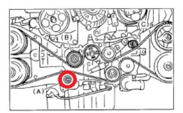
Step 8) Remove the belt idler B and C. The left-hand camshaft sprockets will not rotate.
