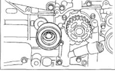
Step 14) Your camshaft sprockets and crankshaft should not have moved since you removed the belt but it is a good idea to double check the marks. The camshaft sprocket double lines should line up with each other on both sides and the single marks should line up with the back side of the timing cover. The crankshaft should line up with the mark on the block.
