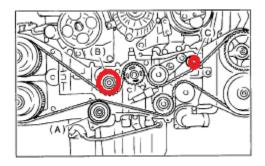
Step 17) Reinstall timing belt guides (manual transmission vehicles). Tighten bolts to 9.8Nm (1.0kgf-m, 7.2 ft-lb)
