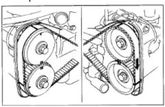
Step 5) For AVCS cam sprockets, remove the cover plates and set aside. Install Company23 Camlock onto left-hand side exhaust and intake camshaft sprockets. If you have intake AVCS cam sprockets only, install spacer on bottom side of the tool between the hex lock pin and the curved tie bar. The tool should be parallel to the cam pulley surfaces.
