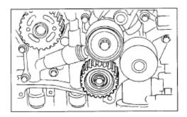
Step 10) Remove the automatic belt tension adjuster.
