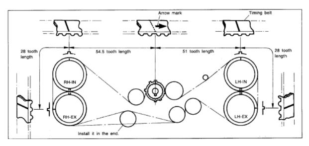
Step 16) Install belt idlers and tighten to 39 Nm (4.0kgf-m, 28.9 ft. lb)
