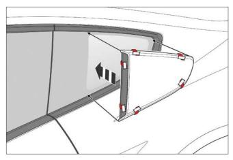
Remove all the tape liners in the order shown below. Be sure to remove the tape liners in the direction indicated.
