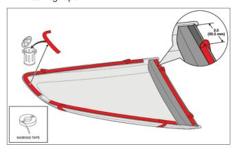
4. Install the window scoop onto the rear quarter glass using the edge of the window's rubber surround molding as a guide. Do not allow the exposed double-sided tape to adhere until the window scoop is properly aligned, then press down.
