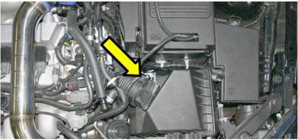
2. Unplug the Mass Air Flow (MAF) harness from the MAF sensor by pushing down on the tab and pulling away from you.
