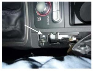
6. (08+ STi Only) Lift up on the rear of the shifter surround and slide it back towards the rear of the car. Unclip the wire underneath this piece in order to be able to set the trim piece aside.
